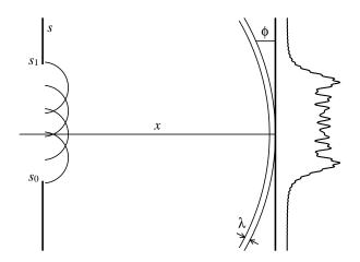
Figure 8: Diffraction through a slit.
