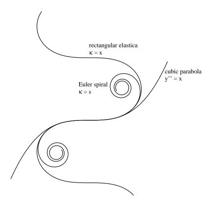
Figure 7: Euler's spiral, rectangular elastica, and cubic parabola.
